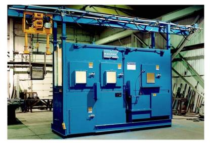
Small, unitized unit with integral handling system for easy installation
