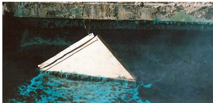
CARC coating being stripped from metal panel
