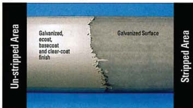
The layers of organic coating have been removed from half of this rail.
