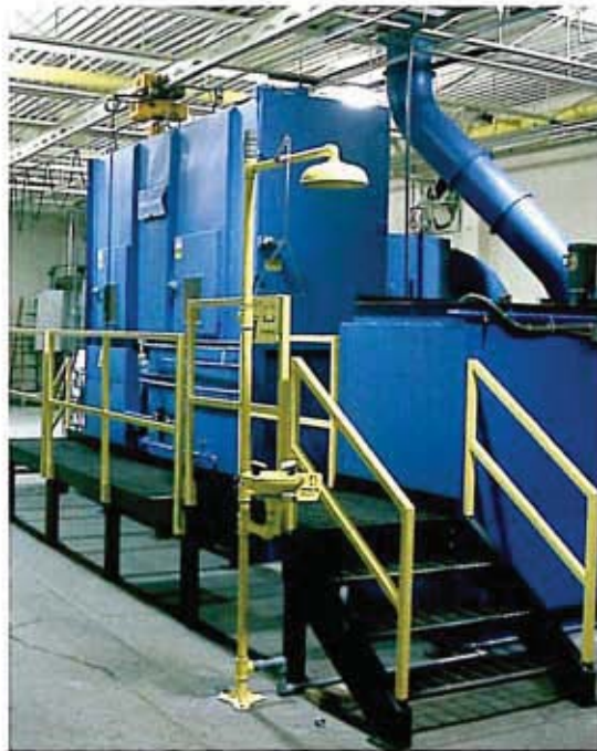
A typical stripping system includes the solution tank and a rinse tank.
