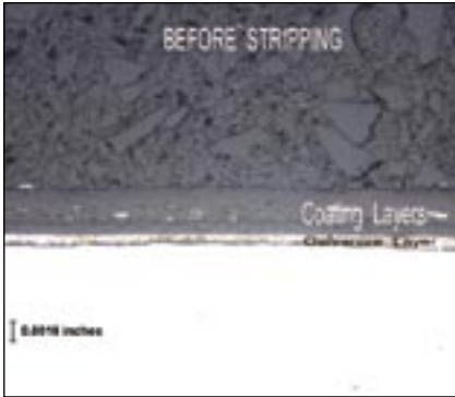
The photomicrograph shows the original coated surface and galvanized layer (left) before stripping, and the unaffected galvanized layer after stripping (right).
