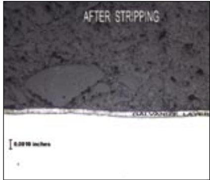
The photomicrograph shows the original coated surface and galvanized layer (left) before stripping, and the unaffected galvanized layer after stripping (right).
